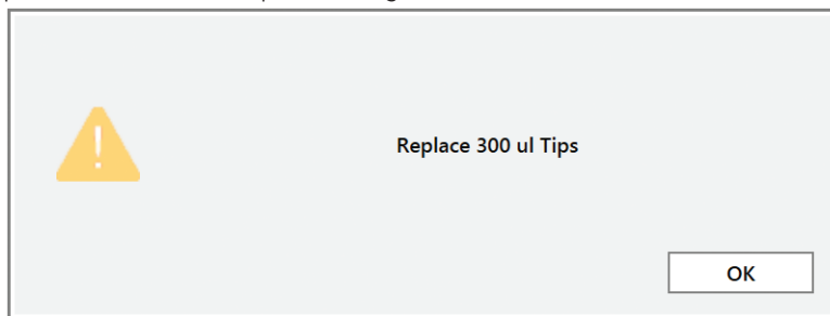
Figure 18. Insufficient tips on the system to complete a method. In the event that all tips of a given tip type are consumed during a run, the instrument will pause and unlock the door. Open the door, load more tips of the indicated type on the tip and plate carrier, close the door and press OK to resume processing.
